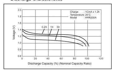
Discharge temperature characteristics at 1lt discharge
