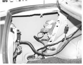
Installation in our 1999 Ford Mustang GT begins with removing the drivers side interior trunk panel to access the fuel pump wiring. Each vehicle model has a specific wire that you'll need to cut, and use for your installation. Ours just happened to be the pink/black wire coming out of the inertia switch and leading to the fuel pump driver. All you do is cut it, and attach the red wire with the fuse from the Boosta-pump to the side that comes from the inertia switch, and
