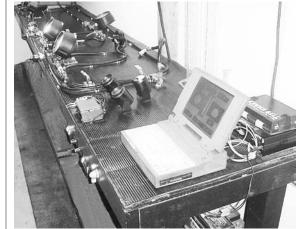
Here is the Kenne Bell Boost a Pump test stand. Bell stands behind all of their products with lots of actual testing, and this test stand helped prove Kenne Bell's theories about the Boost-a-Pump increasing flow without decreasing pump life. It's nice to know that there is actual engineering behind this technology.
