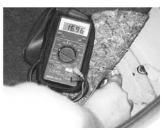
We thought an actual voltage test was in order, so after the installation was complete we started the engine and checked voltage at the fuel pump wire with the variable dash controller all the way at the "0%" position and saw a steady 13.03 volts. This is actually better than most stock wiring, as most we've tested are in the 11.8-12.8 volt range in stock configuration. After turning our dash mounted variable controller all the way up to the "50%" setting on the knob, we immediately saw our volt
