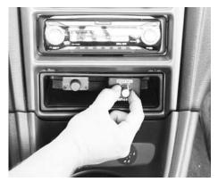
We mounted our BAP knob right under our stereo—that way we can make quick adjustments if we need to at the dyno or on the track.
