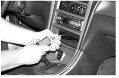
After getting the wiring to the front of the car, we ran the RCA type connector for the dash mounted variable controller through a hole we drilled in the rear of the empty pocket underneath the radio. At this point, just plug it in to the back of the variable controller and mount it. We used some really sticky 3M two sided tape and stuck it to the inside of the pocket.
