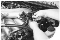
The activation switch (boost or vacuum) gets a pair of wires hooked to it. In our application, we used the boost pressure switch and tee'd it off a vacuum fitting. There is no polarity on the two wires that you hook to the switch, just plug them in and tuck it all out of sight. While it is possible to simply twist these two wires together and have the Boosta-pump activated at all times without any harmful recourse, Mr. Bell sees no
